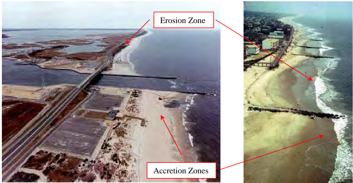
Images depicting impact of manmade structures (jetties and groins) on near shore sediment transport Modified images from http://www.ocean.udel.edu/mas/wcarey/monthlyquestions/april04.html
